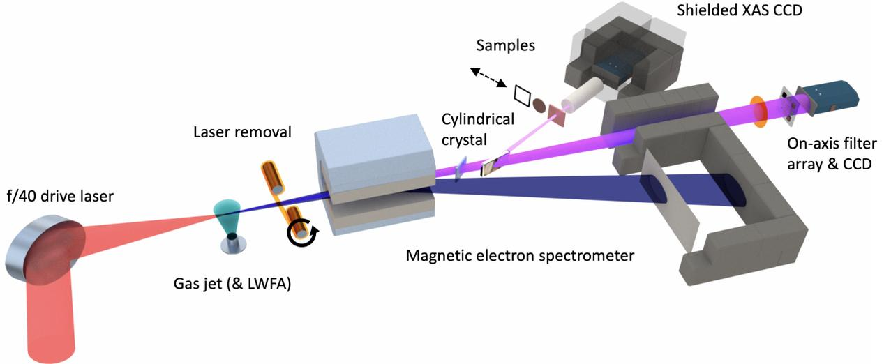
Figure 1: Overview of the experimental setup. An  $f/40$  laser creates a LWFA in a high pressure gas jet, generating a beam of on-axis electrons and x-rays. The electrons are swept away by a dipole magnet and the x-rays are either diffracted off a cylindrical crystal through a sample and spectrally spread onto a shielded CCD, or alternatively (with the crystal translated out) straight onto a CCD through a multi-element filter array used to infer the broad spectral shape.
