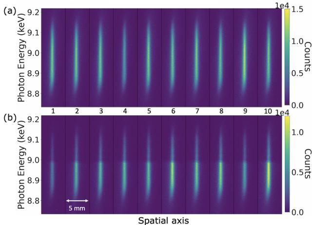
Figure 2: (a) Raw XAS CCD data for ten consecutive shots. The x-rays are spatially focused to a line, and spectrally spread in the vertical axis. (b) The next 10 consecutive shots, but with a  $4 \mu\text{m}$  copper foil placed in the x-ray beam. The K-edge absorption is clear, and the LWFA x-rays are performing in a stable manner.
