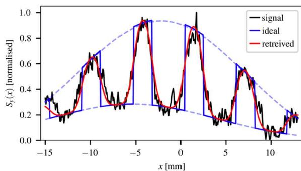
**Figure 2:** Example signal modulation fitting for beam parameters retrieval. The signal (black line) is taken for a central positron energy of 420 MeV with a converter thickness of 8 mm. An ideal beam (zero source size) would produce a rectangular profile pattern (blue line) between the scattered signal and the beam amplitude (blue dashed lines). Deviations from this ideal behaviour allow one to extract the beam source size.
