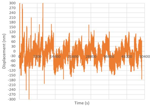
Figure 11: A 13.5 hour test showing stability before the motion control was tuned (30 nm = 0.1 μrad)
