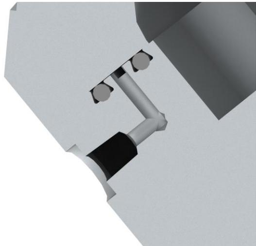
Figure 4: Cross-section through differentially pumped seal
