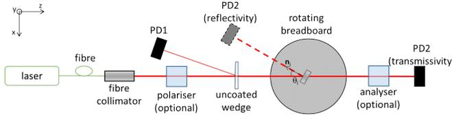
Figure 1: *Experimental setup for the room temperature beamline of CARAVAGGIO.*
