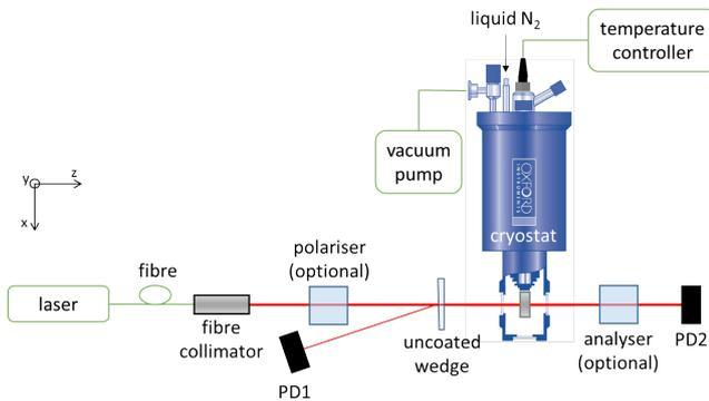
Figure 2: *Experimental setup for the optical cryostat beamline of CARAVAGGIO.*
