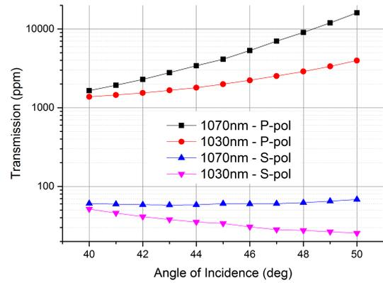
Figure 3: *Experimental results for a rectangular mirror, obtained using the room temperature CARAVAGGIO beamline. The scale is logarithmic in order to fit all results in a single graph.*
