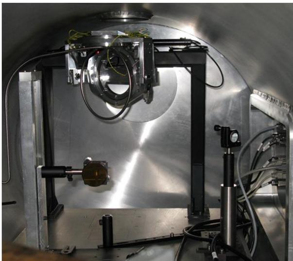
*Figure 3. The new G1 mount in place in the chamber, without the grating. The antenna for RF cleaning can be seen in front of the mount. The back mirror and its mount fit on the back of the breadboard behind the black frame.*
