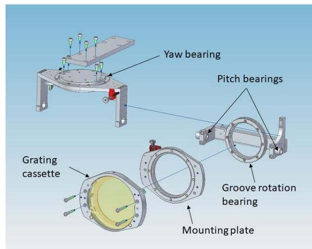
Figure 1. Exploded CAD diagram of the new mount showing the key components and their relationship
