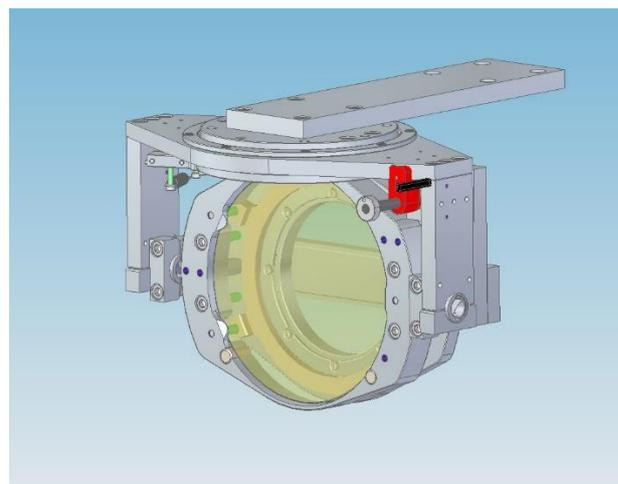
Figure 2. CAD drawing of the assembled grating mount
