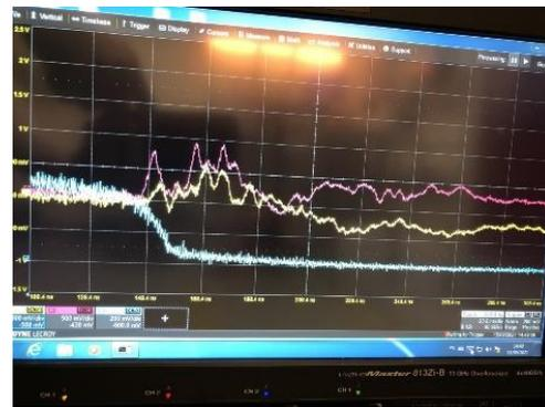
Figure 7: B-Dot, D-Dot Probe traces
