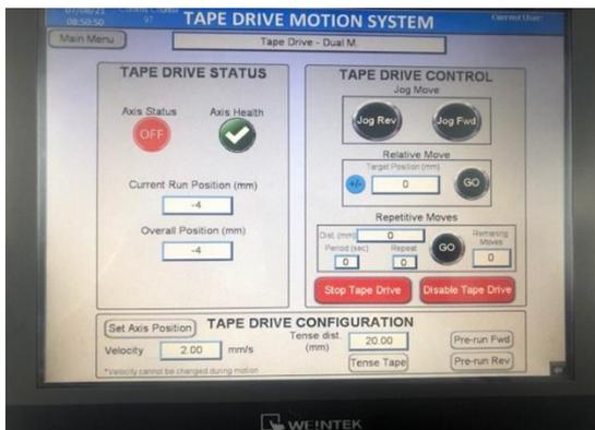
Figure 5: Tape Drive Control Software on the HMI
