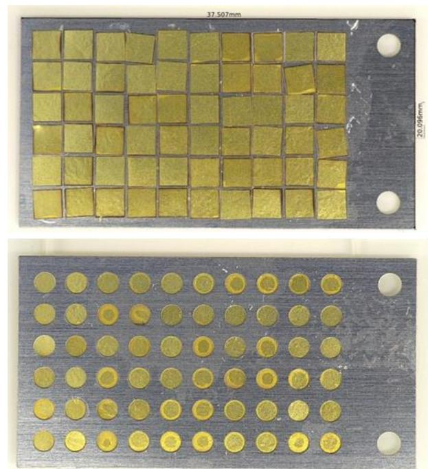
Figure 5: (top) Upper side of target array with sixty 2.8 mm square gold foil targets that are 30  $\mu\text{m}$  thick; (bottom): Laser-facing side of (same) target array
