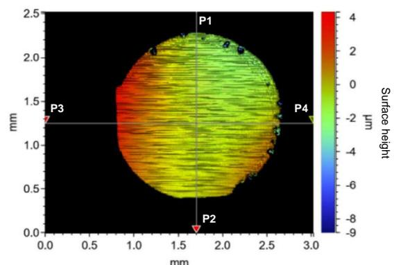
Figure 6: Foil position and topography of a single aperture in an assembled target array (from laser-facing side)
