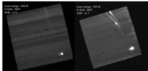
Figure 2: Images from lanex, before shielding (left) and after full shielding (right).
