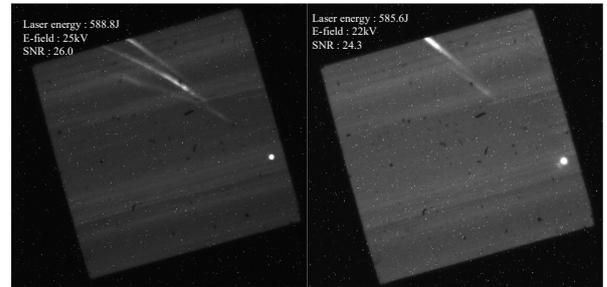
Figure 5: Best comparison between gadox(left) and lanex(right).
