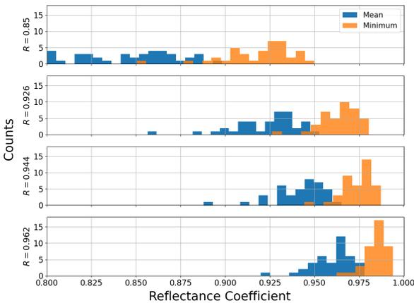
Figure 5: Distribution of effective reflectance coefficients from Dasgupta et. al’s report, where each row signifies where the minimum (green) or mean (blue) reflectance coefficient corresponding to Dasgupta’s data points. All data points satisfy the condition  $R < 1$ .
