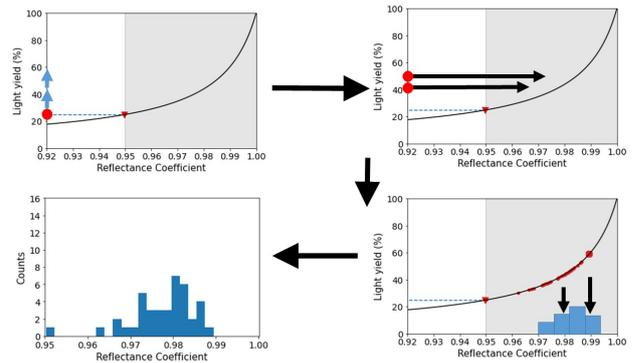
Figure 3: Graphical representation of the light yield model being used to find the effective reflection coefficients of each data point.
