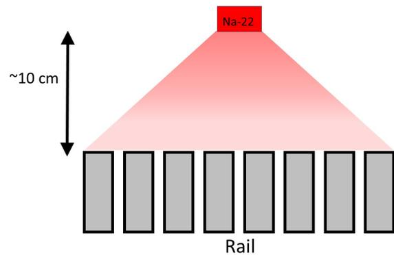
Figure 1: Calibration setup of X-ray spectrometer. The distance of the radiative source was much larger than the width of the rail, and so the amount of radiation incident on each block can be considered uniform.
