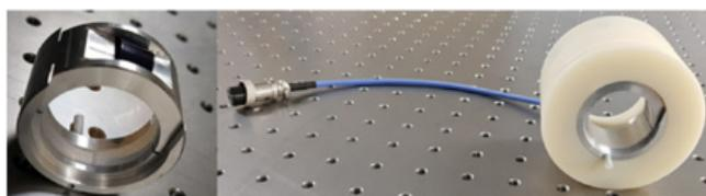
Figure 3: Photographs of LBO crystal oven components: (left) spring-loaded metallic crystal holder with the crystal in place. This is placed inside the oven unit (right). The oven is then connected to a separate temperature control unit.
