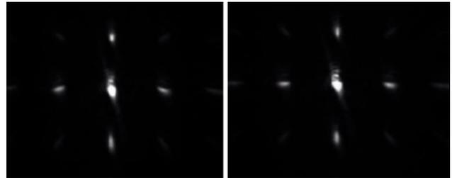
Figure 2: Angular dispersion (AD) diagnostic camera images of undeviated (left) and optimised (right) pulse
