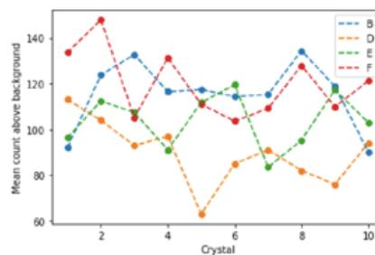
Rail calibration schematic (left) and results (right) demonstrating high variability in uniform set of crystals. Subtle variation in average reflective coefficient can explain the measured variation in yield.
