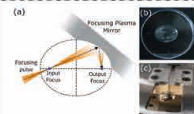
(a) Illustration of ellipsoidal focusing plasma mirror concept. Images of (b) the manufactured diamond machined optic and (c) the injection moulding tool.
