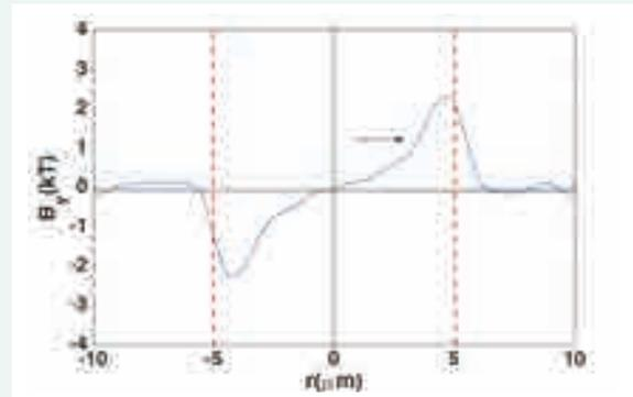
Cross-section of the magnetic field,  $B$ , as a function of radial position  $r$  at  $x=10 \mu\text{m}$ , taken at  $2.2 \text{ ps}$  and limited to  $-10 < r < 10 \mu\text{m}$  in  $y$ -midplane. The vertical dashed lines show the boundaries of the guide element. The arrow shows the gradient in the magnetic field inside the guide-element.
