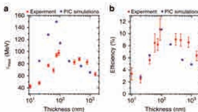
(a) Proton maximum energy scaling and (b) conversion efficiency scaling with target thickness.
