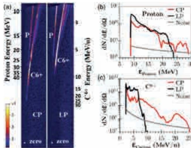
(a) Raw data from BAS-TR image plates for CP and LP laser pulses irradiating 10 nm amorphous carbon targets. The corresponding CP (red) and LP (black) background-subtracted proton (b) and  $\text{C}^{6+}$  spectra (c) with vertical axis units of particles/MeV/sr are also shown. The noise level of  $+2\sigma$  is also plotted.
