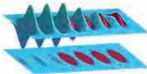
Model of a train of pulses (in red) used to drive a plasma wave (in blue).
