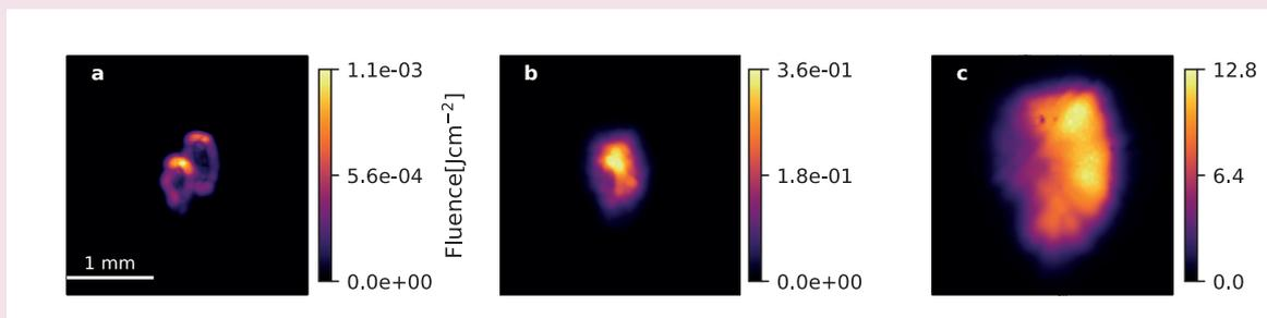
Transverse profile of the Raman signal. Recorded beam profiles for three different nominal pump energies: (a) 3 J, (b) 20 J, (c) 70 J.
