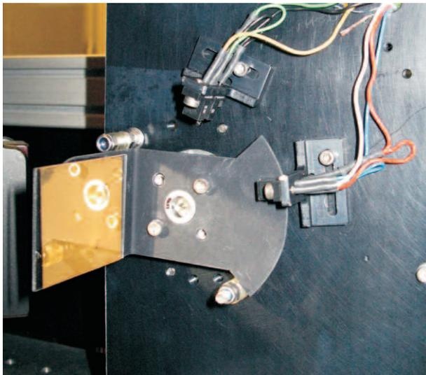
**Figure 1.** Low inertia blade with gold reflector capable of selecting a single 10 Hz pulse.
