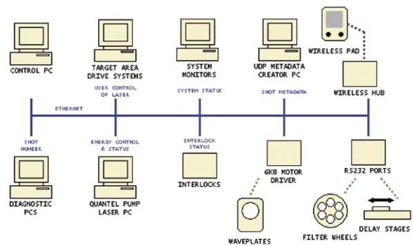
**Figure 3.** Gemini Control Network. The Ethernet has become a straightforward way to connect remote controllers and hardware to the control PC.
