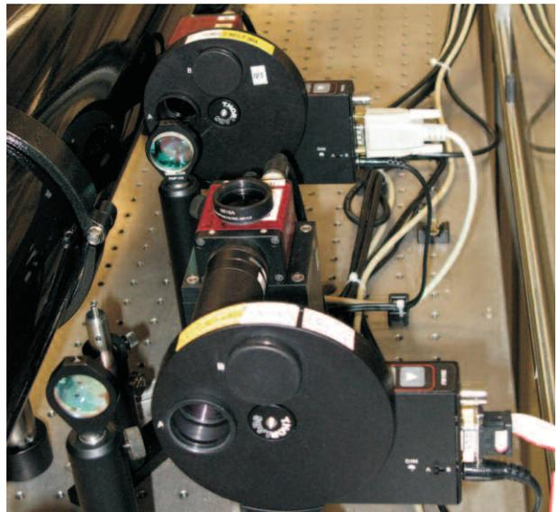
**Figure 2.** Filter wheels installed to automatically attenuate pulse on high power shots.
