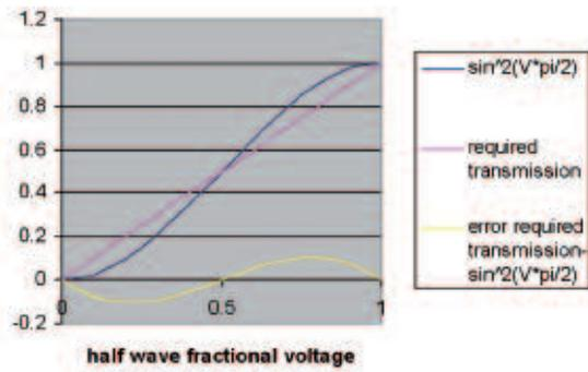
Figure 3. Fractional transmission error.
