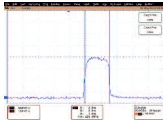
Figure 8. Corresponding 4 ns 213 J output on Beam 7 delivered to TAE.
