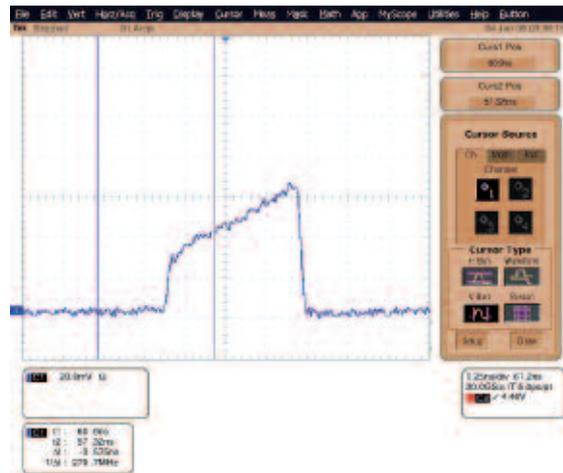
Figure 7. Corrected 4 ns linear optical ramp from oscillator.
