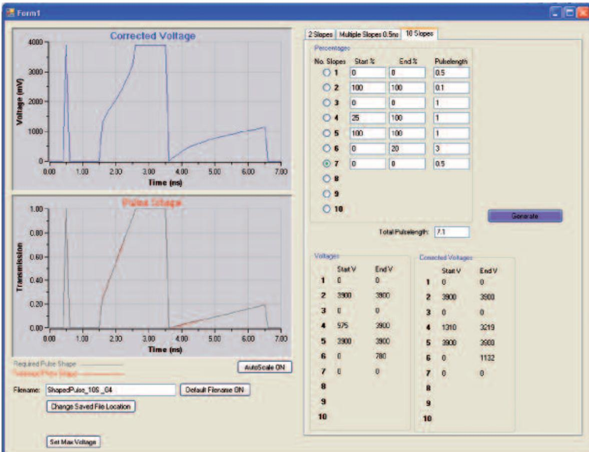
Figure 4. AWG text file generation programme for an example shape. Corrections for ramp outputs require ‘close to parabolic’ voltage corrections.
