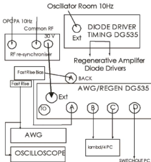
Figure 1. Timing scheme for the AWG and regenerative amplifier for Vulcan synchronization.
