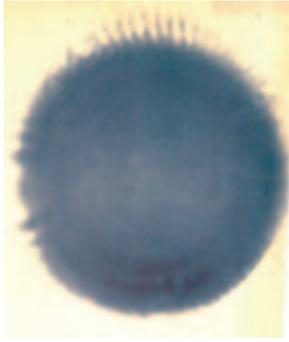
Figure 6. Transverse spatial profile of full energy shaped pulse.
