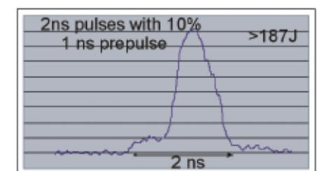
Figure 2. Examples of full energy shaped long pulses delivered on Beam 6 during commissioning work.
