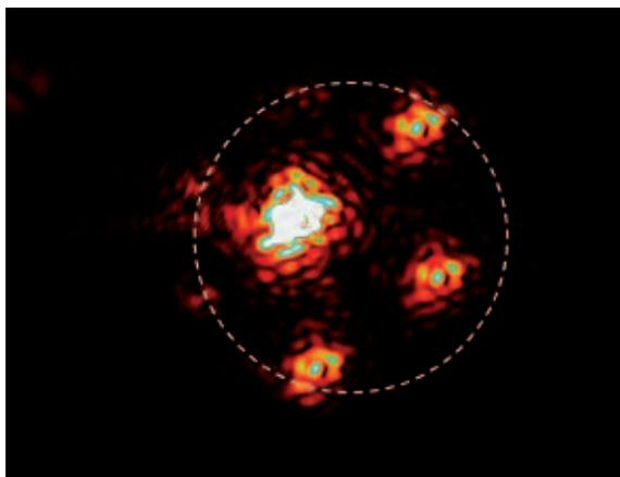
Figure 4. The diffraction spot pattern visible for a misaligned beam, some of the pattern is obscured by the pinhole. The dashed line shows the approximate pinhole size and position.
