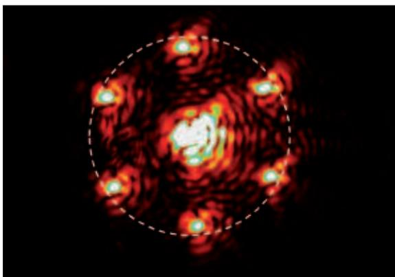
Figure 2. The diffraction spot pattern generated at focus. The dashed line shows the approximate pinhole size.
