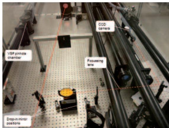
Figure 3. A view of the optical layout looking down from above the amplifier.
