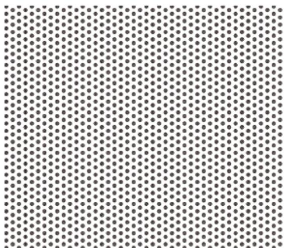
**Figure 1.** An example of an amplitude mask which creates a hexagonally symmetric diffraction pattern at focus.
