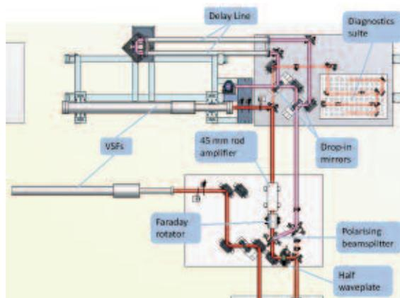
Figure 2. The optical layout: Beam 8 is shown in red, beam 7 is shown in pink. The diagnostics channel for beam 8 is shown as a dashed line (the beam 7 diagnostics are not visible in this view as they are on the lower level beneath the table).
