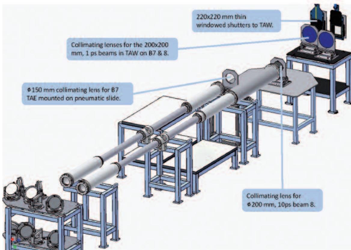
Figure 3. A 3D CAD image of modifications to beam lines 7 and 8 in laser area 3.
