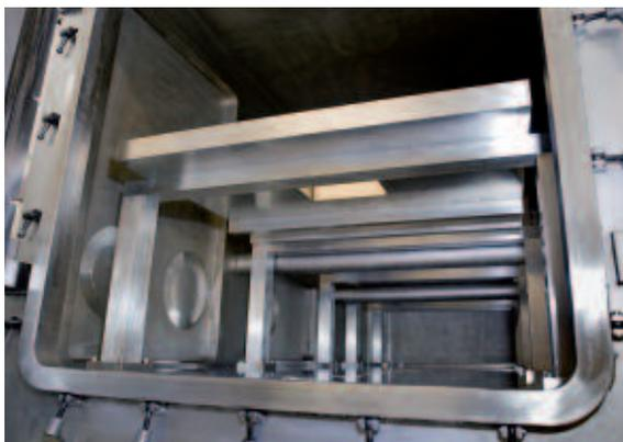
**Figure 4. Reinforcement elements under upper breadboard.**
