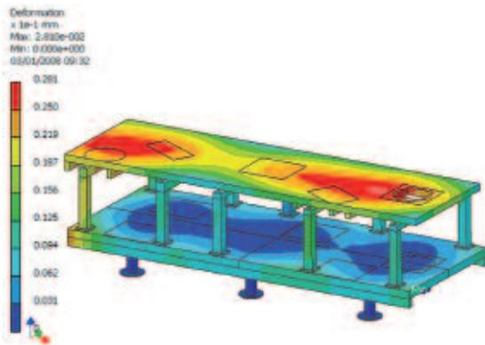
Figure 8. FEA map of calculated deformations.
