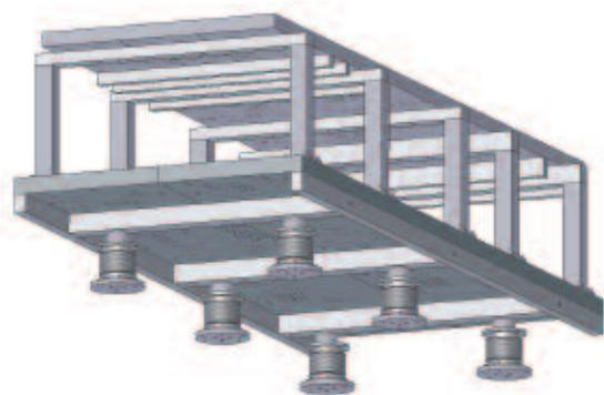
**Figure 6. Lower breadboard reinforcement bars and support columns.**
