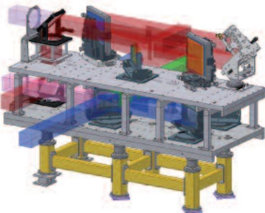
Figure 1. 3D model of support frame with optical mounts.
