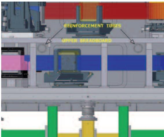
**Figure 3. Model of support frame inside compressor chamber showing position of reinforcement tubes and optical mounts.**
