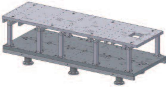
Figure 7. 3D model of support frame in its final design.
