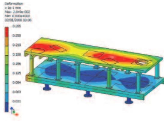
Figure 9. FEA map of calculated deformations – one of the grating mounts is at a different position.
