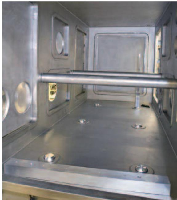
Figure 2. Reinforcement tubes inside compressor chamber.
